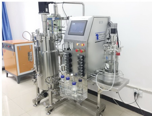
BLBIO-5GJ-50SJ 5L-50L Secondary Fermentation System
