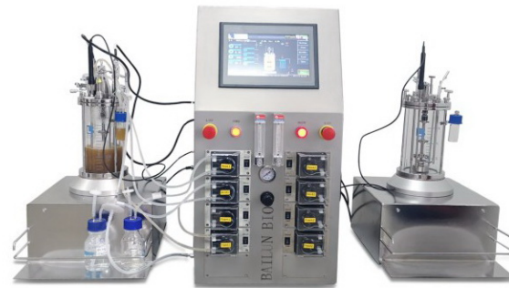
BLBIO-XGC-2-A Double magnetic mixing glass fermenter (desktop)
