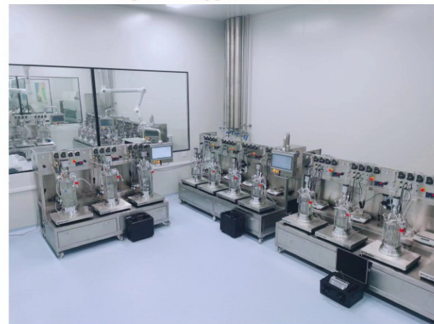
BLBIO-XGJ-11-plus Elevenfold mechanical mixing glass fermenter (5L)
