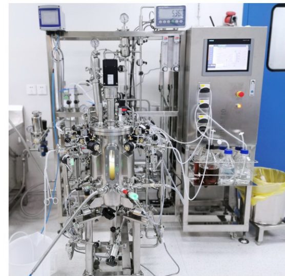
BLBIO-30SJA-FMT 30L Metabolic flow automatic bioreactor system
