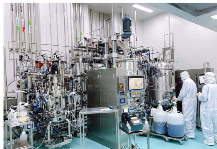
50L-800L Top magnetic mixing bioreactor
