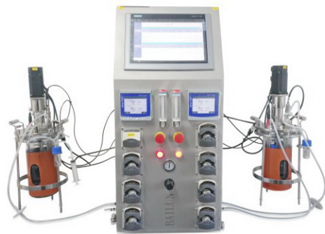
BLBIO-XGJG-2-A Double mechanical mixing single wall glass fermenter (desktop)
