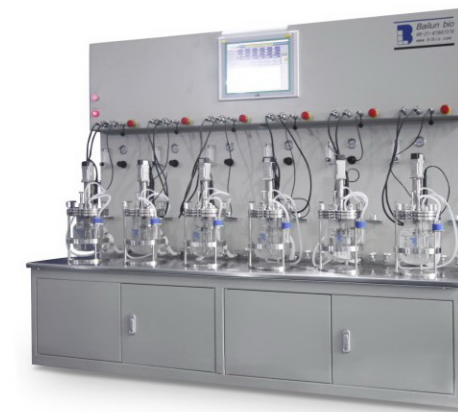
BLBIO-XGJGG-6 Sextuple double wall glass fermenter (2L)
