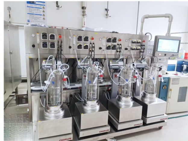
BLBIO-XGC-4-plus Quadruple magnetic mixing glass fermenter (5L)
