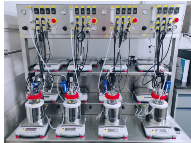
BLBIO-XGC-4-plus Quadruple mechanical mixing glass fermenter (500mL)
