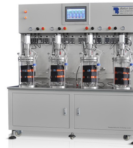
BLBIO-XGJG-4-H Quadruple mechanical mixing single wall glass fermenter (5L)
