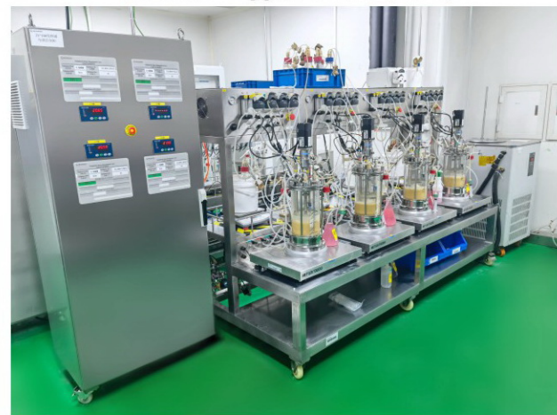
BLBIO-XGJ-4-plus Quadruple mechanical mixing glass fermenter (5L)
