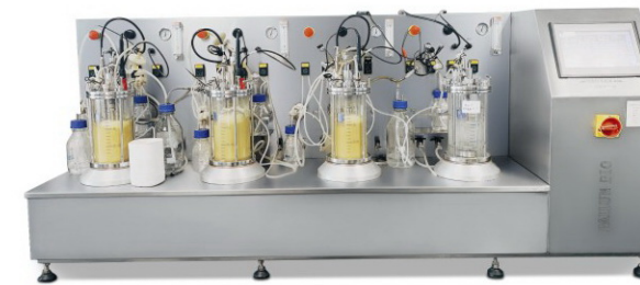
BLBIO-XGC-4-H Quadruple magnetic mixing glass fermenter (5L)
